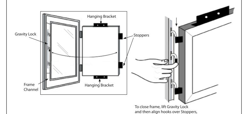
then release Gravity Lock to secure
